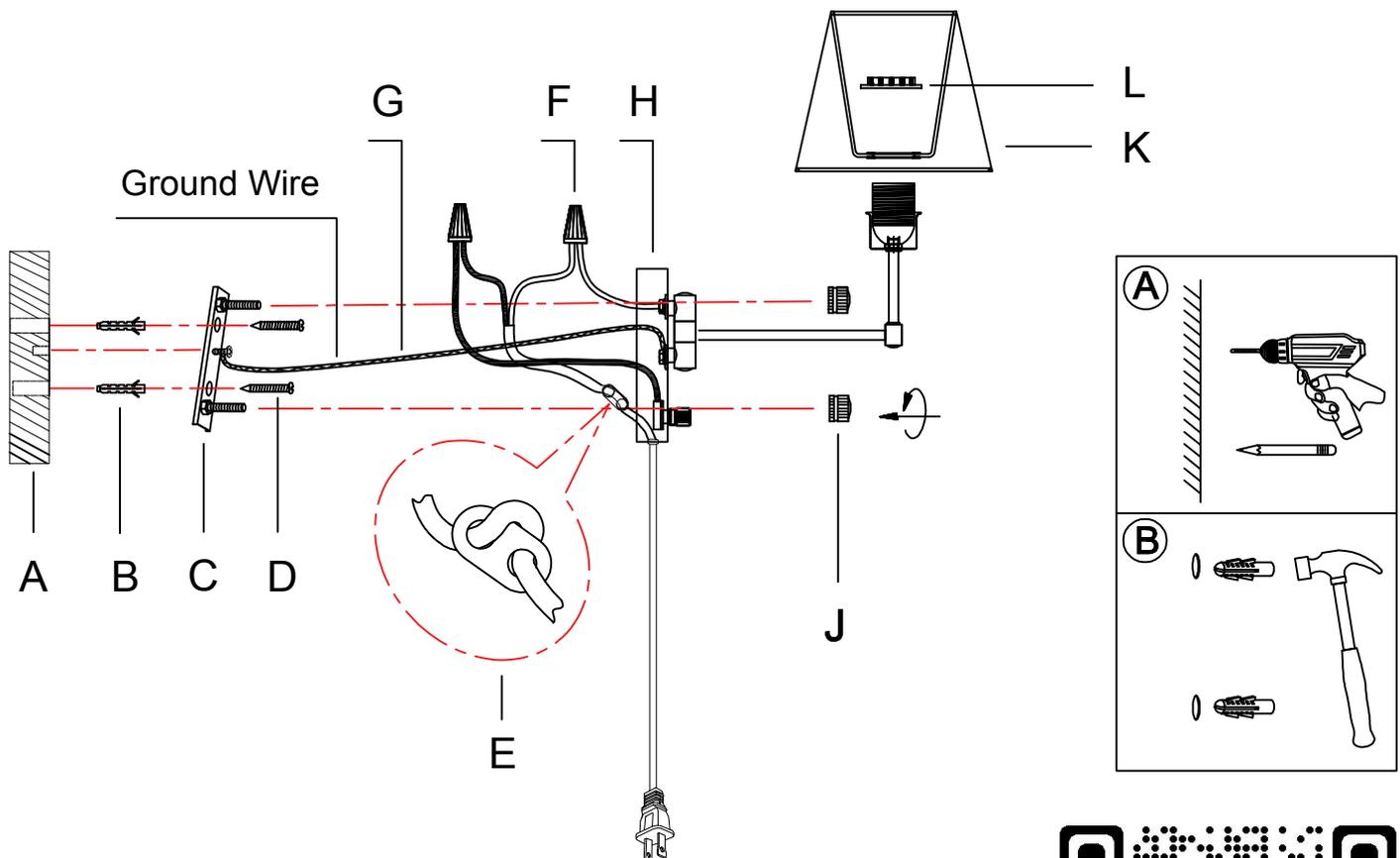
Note: The way to differ the neutral wire from the live wire is that a white line is printed on the cover of the neutral wire .
