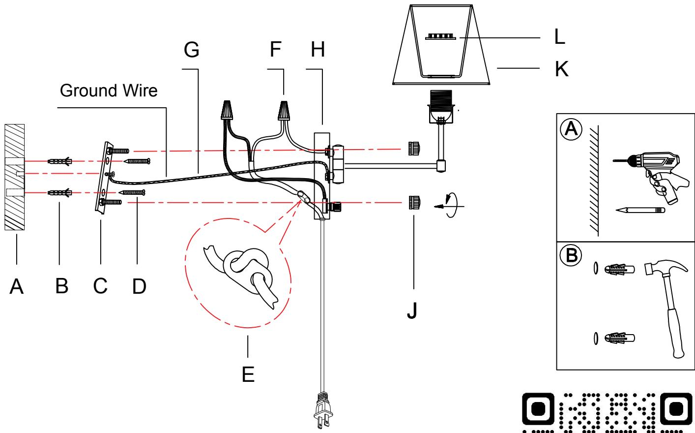
Note: The way to differ the neutral wire from the live wire is that a white line is printed on the cover of the neutral wire .
