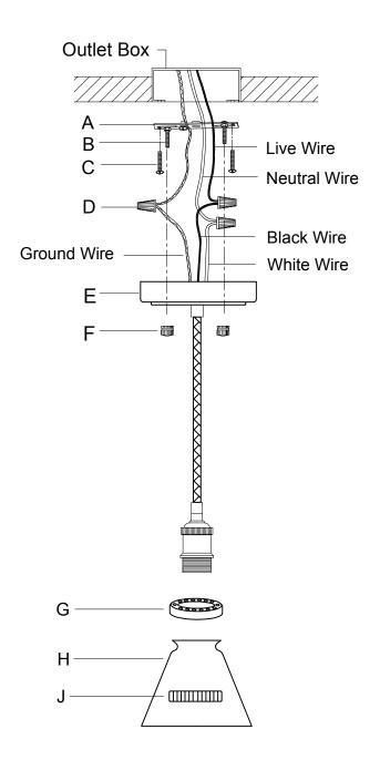
In view of thermal expansion and contraction, avoid securing the glass shade too tight when screwing the socket ring into the lamp holder, or you will break the glass shade.
