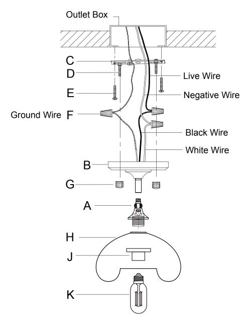
In view of thermal expansion and contraction, avoid securing the glass shade too tight when screwing the socket ring into the lamp holder, or you will break the glass shade.
