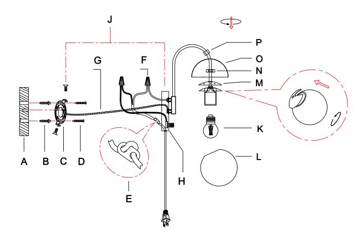
Note: The way to differ the neutral wire from the live wire is that a white line is printed on the cover of the neutral wire .
