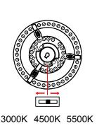
The LED color temperature can be adjusted before installing the lamp.
