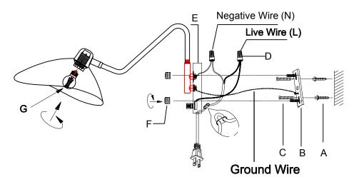
Note: The way to differ the negative wire from the live wire is that a white line is printed on the cover of the negative wire.
