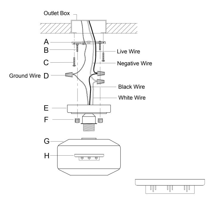
Note: Always keep the bigger side of the socket ring on top when screwing the socket ring into the lamp holder. In view of thermal expansion and contraction, avoid securing the glass shade too tight when screwing the socket ring into the lamp holder, or you will potentially break the glass shade.
