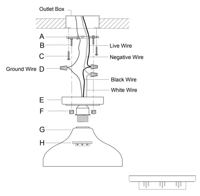
Note: Always keep the bigger side of the socket ring on top when screwing the socket ring into the lamp holder. In view of thermal expansion and contraction, avoid securing the glass shade too tight when screwing the socket ring into the lamp holder, or you will potentially break the glass shade.
