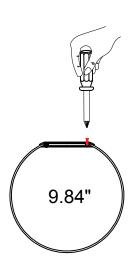
Tighten the screws before installing the glass globe. Note: Do not over tighten the screws or you will potentially break the glass.
