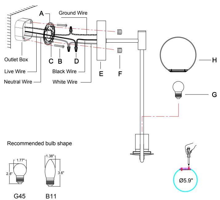
Max. Size of Bulb: 1.77 Inches Width \* 3.6Inches Height Tighten the screws before installing the glass globe. Note: Do not over tighten the screws or you will potentially break the glass.
