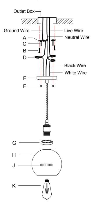
In view of thermal expansion and contraction, avoid securing the glass shade too tight when screwing the socket ring into the lamp holder, or you will break the glass shade.
