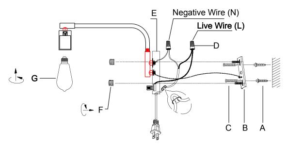
Note: The way to differ the negative wire from the live wire is that a white line is printed on the cover of the negative wire.
