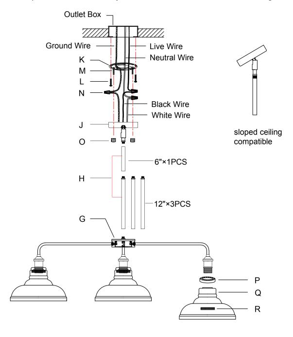
In view of thermal expansion and contraction, avoid securing the glass shade too tight when screwing the socket ring into the lamp holder, or you will break the glass shade.
