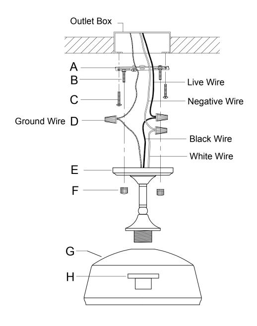
Note: Always keep the bigger side of the socket ring on top when screwing the socket ring into the lamp holder. In view of thermal expansion and contraction, avoid securing the glass shade too tight when screwing the socket ring into the lamp holder, or you will potentially break the glass shade.
