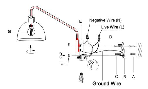
Note: The way to differ the negative wire from the live wire is that a white line is printed on the cover of the negative wire.
