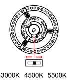
The LED color temperature can be adjusted before installing the lamp.
