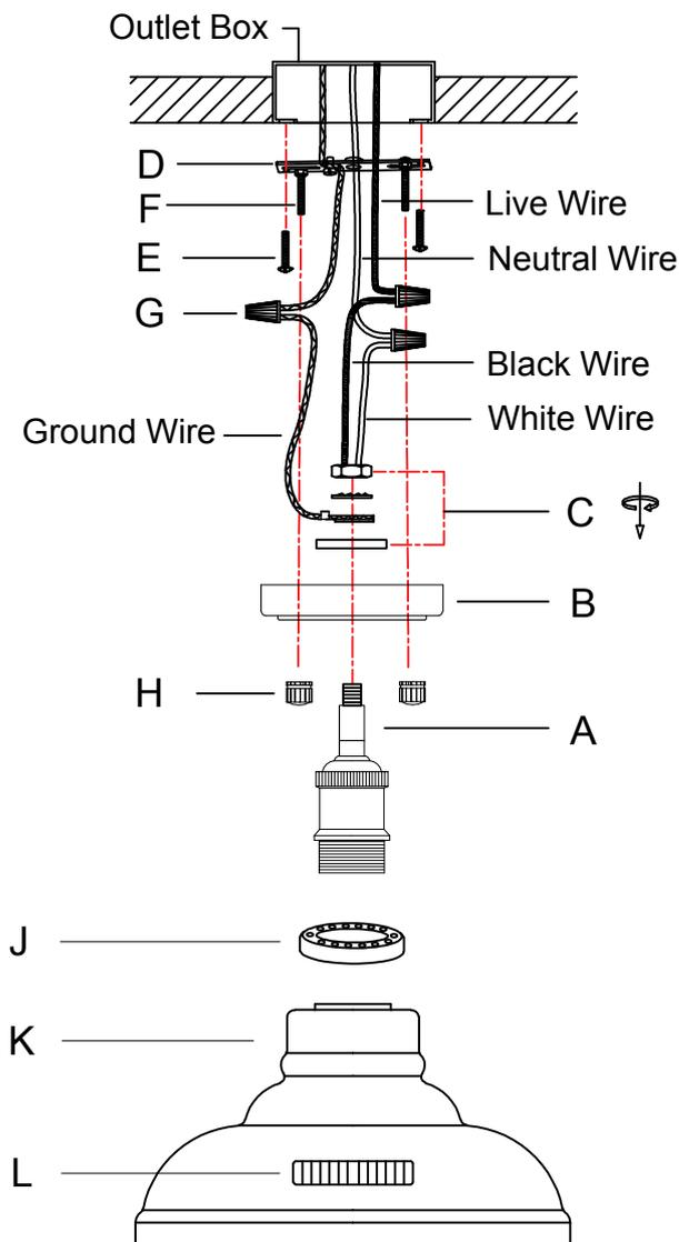
In view of thermal expansion and contraction, avoid securing the glass shade too tight when screwing the socket ring into the lamp holder, or you will break the glass shade.
