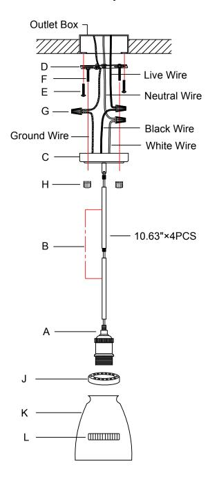
In view of thermal expansion and contraction, avoid securing the glass shade too tight when screwing the socket ring into the lamp holder, or you will break the glass shade.
