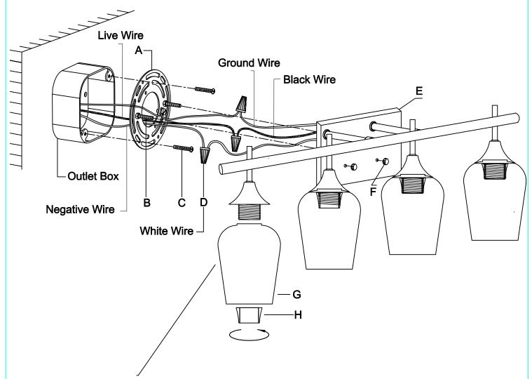
In view of thermal expansion and contraction, avoid securing the glass shade too tight when screwing the socket ring into the lamp holder, or you will break the glass shade.
